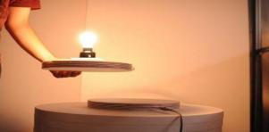
magnetic field. Once an RX (Receiver) coil is located near to the magnetic field, then the magnetic field can induce an AC current in the receiving coil. Electrons in the receiving device, converts the AC current back into DC current that becomes working power.
