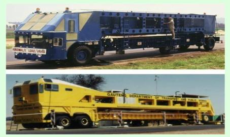
The HVS-Airfield Mk V at WES is typically used for high wheel load short duration APT studies.
