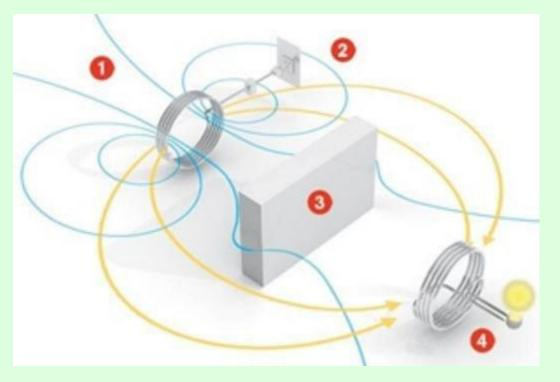
The basics of wireless power transmission include the inductive energy that can be transmitted from a transmitter coil to a receiver coil through an oscillating magnetic field. The DC current supplied by a power source is changed into high frequency AC current by particularly designed electronics built into the transmitter.
